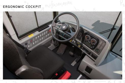
Every bus driver is different. The offset gauge cluster and the optional adjustable pedals make driving easier and safer for drivers of every shape and size. The standard tilt/telescoping steering wheel makes driving more comfortable for drivers.
